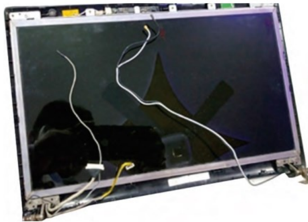
Fig. 2.24: Separate LCD screen from back cover
