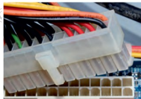
Fig. 1.44: Unplug 20-pin ATX
