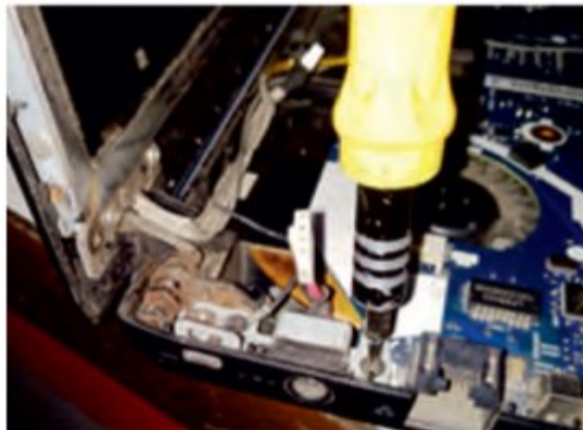
Fig. 2.15: Open the hinge and remove DC power jack
