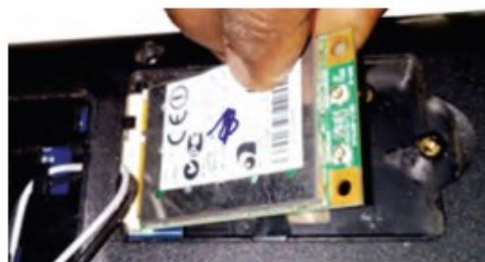
Fig. 2.17: Disconnect Wi-Fi Module
