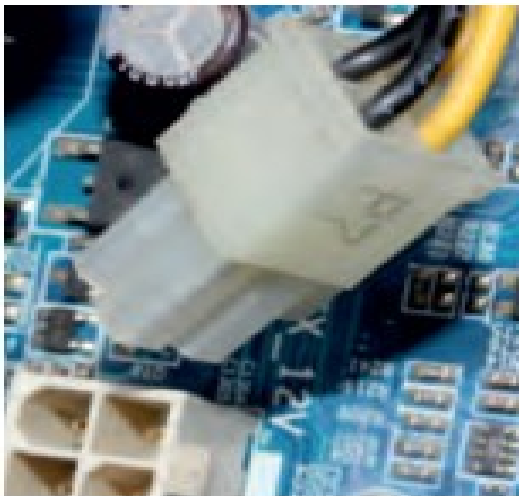
Fig. 1.45: unplug 4-pins AUX power connector from power connector from motherboard
