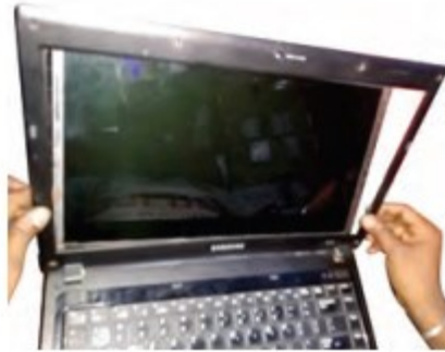
Fig. 2.21: Notebook PC LCD screen removal
