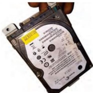
Fig. 2.9: Remove hard drive assembly Fig. 2.10: Disconnect SATA cable
