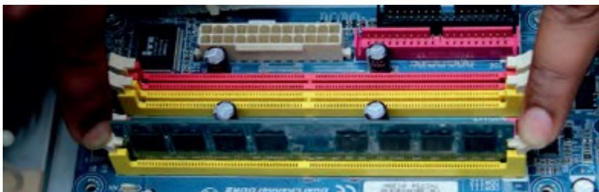
Fig. 3.12 Press down the memory in slot
