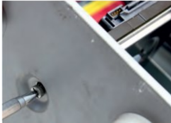
Fig. 1.50: Unscrewing of HDD
