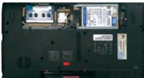
Fig. 2.7: Remove screw from the hard drive and disconnect it
