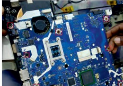
Fig. 2.18: Disconnect cable from motherboard and remove screws
