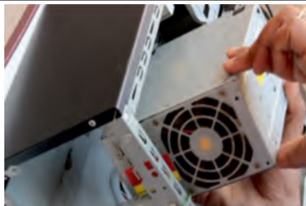
Fig. 1.4: Insert power supply
