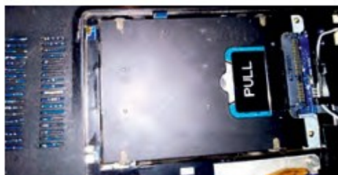
Fig. 2.8: Open the connector and release hard drive cable
