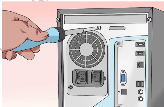
Fig. 1.5 Insert the PSU
