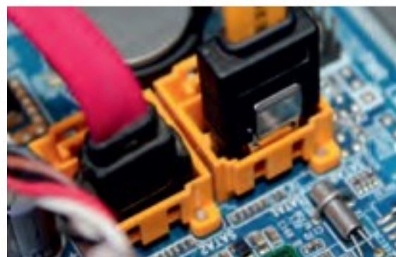
Fig. 1.46: Unplug SATA cables from motherboard
