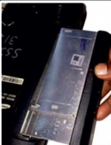
Fig. 2.13: Remove optical CD DVD drive connector board
