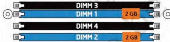
Fig. 3.8: Dual-channel with two DIMMs
