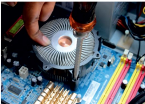
Fig. 1.43: Unscrew heat sink
