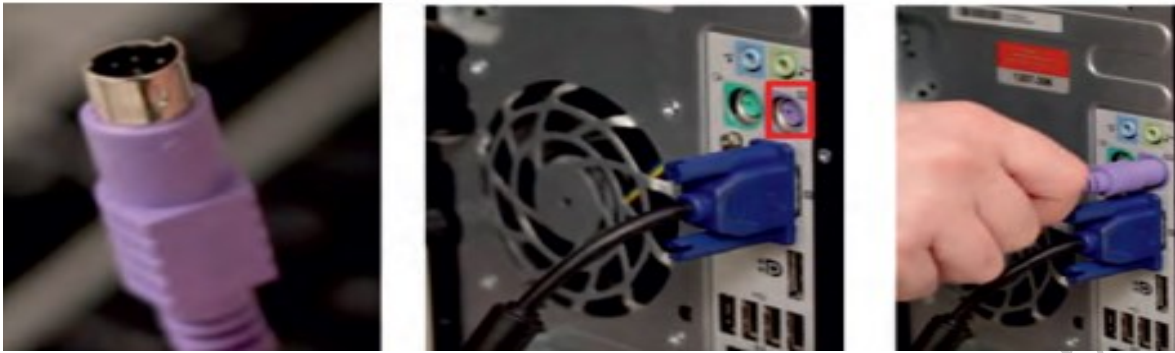
Fig. 1.23: Connecting keyboard in PS/2 port
