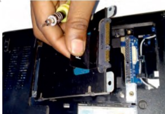
Fig. 2.9: Remove hard drive assembly Fig. 2.10: Disconnect SATA cable
