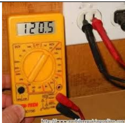
Fig. 3.12: Measurements of AC Voltage
