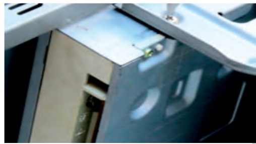
Fig. 1.15: Tighten screws of optical drive
