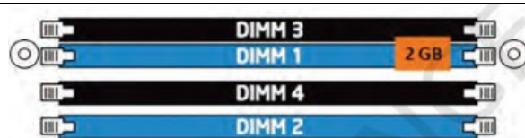
Fig. 3.7: Single-channel with one DIMM
