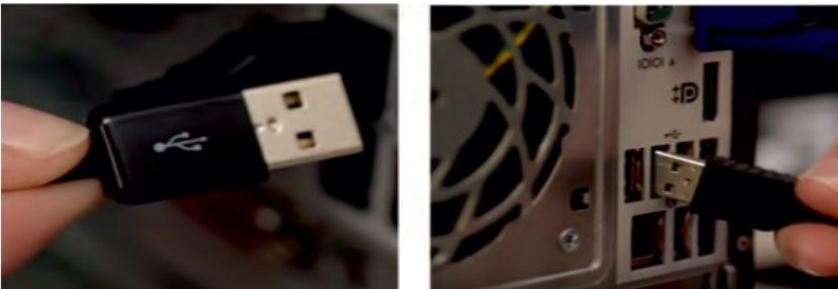
Fig. 1.24: Connecting keyboards in USB port
