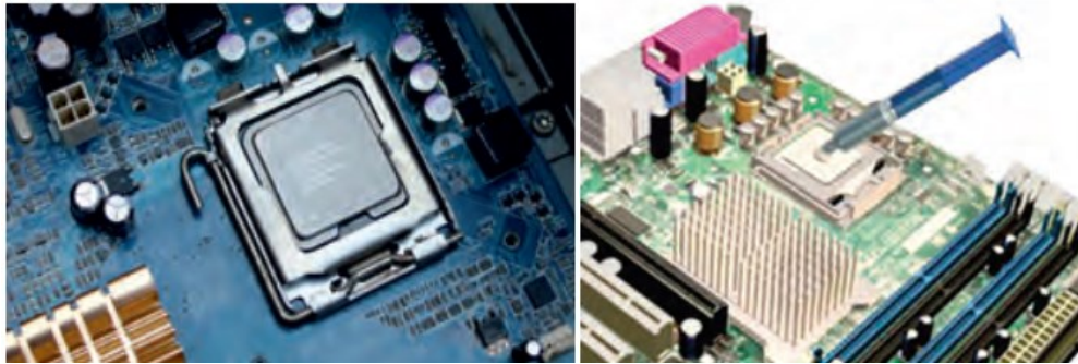
Fig. 2.9 Installing CPU on the motherboard Fig. 2.10 Applying thermal compound on CPU CPU heat sink
