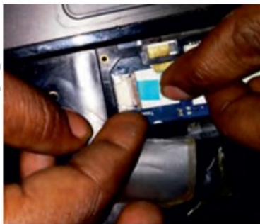
Fig. 2.20: Keyboard permanently attached to top case
