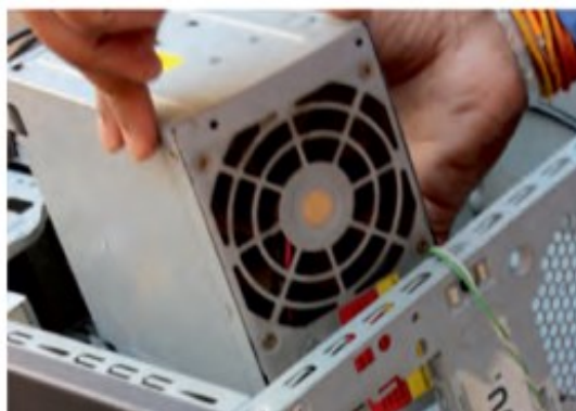
Fig. 1.49: Unscrew the SMPS and remove it from cabinet
