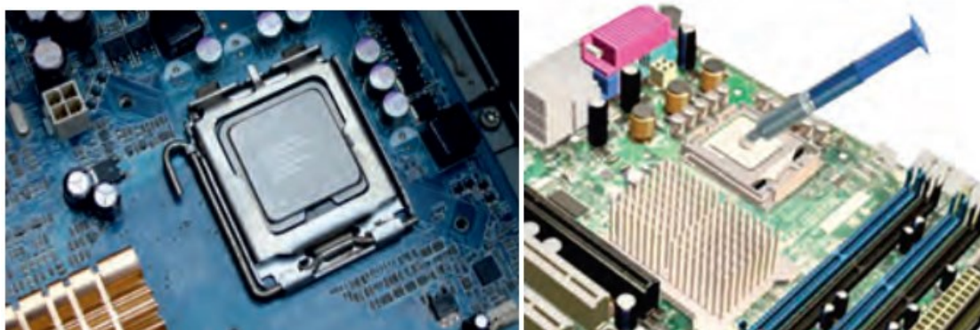
Fig. 1.5: Installing CPU on the motherboard Fig. 1.6: Applying thermal compound on CPU
