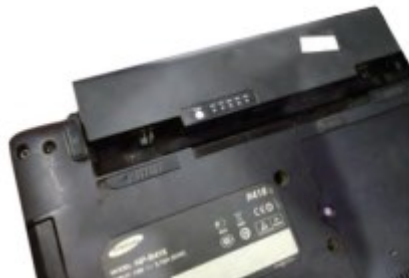
Fig. 2.5: Remove battery and optical drive
