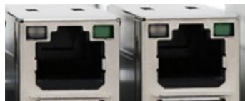
Fig. 1.47 Ethernet or a LAN port with 8P – 8C type connector
