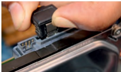
Fig. 1.16: Connect cable IN to HDD
