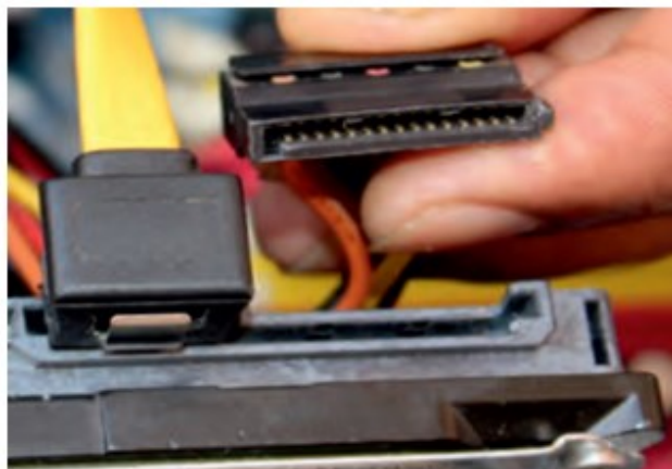
Fig. 1.39: Unplug 15-pin connector from HDD
