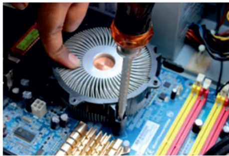
Fig. 2.12 Screwing the heat sink
