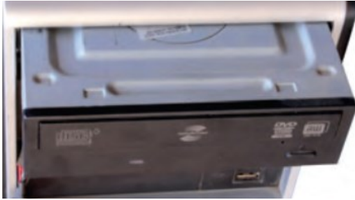
Fig. 1.14: Insert optical drive
