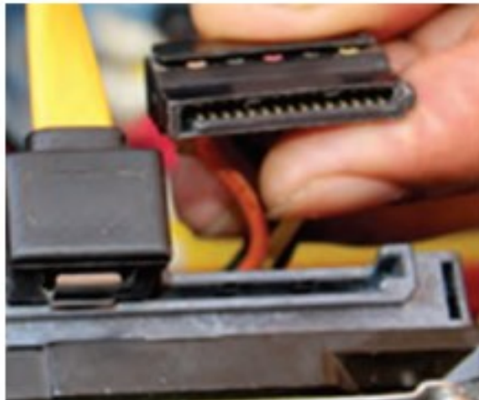
Fig. 1.47: Unplug power cable from optical drive and HDD
