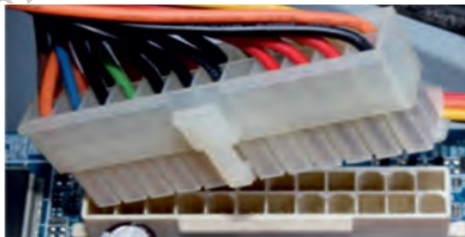
Fig. 1.18: Plug-in 20-pin ATX power connector to motherboard
