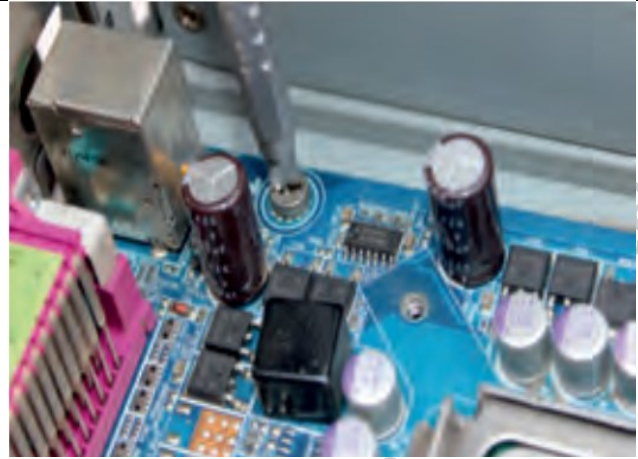
Fig. 1.10: lay the motherboard over the standoffs Fig. 1.11: Tighten all the motherboards screws
