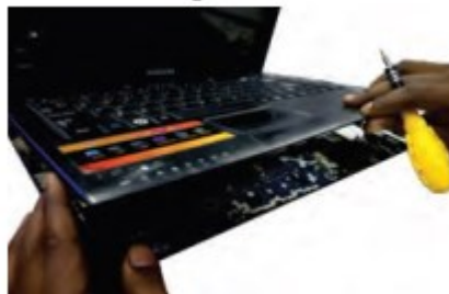
Fig. 2.6: Separate palm rest from bottom case
