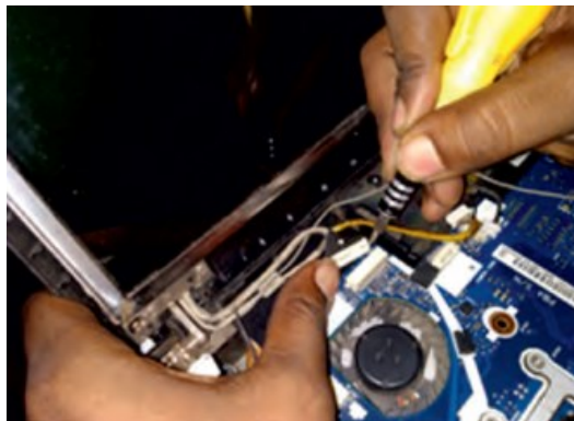
Fig. 2.25: Disconnect video cable from screen
