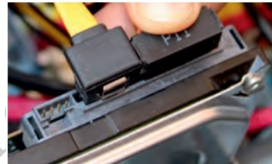
Fig. 1.17: Press cable socket for proper connection
