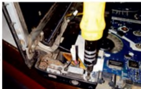
Fig. 2.16: DC power jack mounted under display hinge
