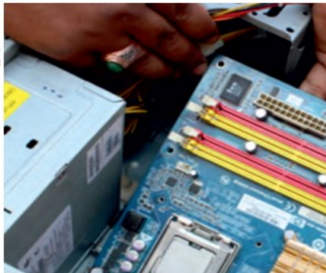
Fig. 1.54: Removing the motherboard
