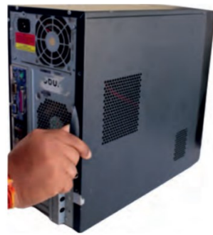
Fig. 1.2: Pull cabinet side cover
