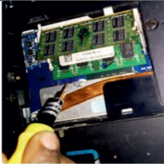
Fig. 2.11: Remove RAM memory modules
