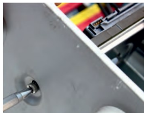
Fig. 1.13: Tighten screw of HDD
