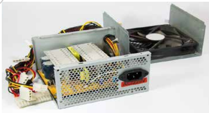
Fig. 2.12 Interior view of a PSU
