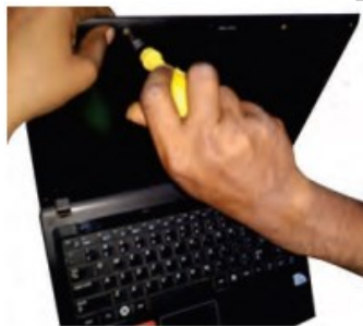
Fig. 2.22: Remove the four screws securing LCD screen
