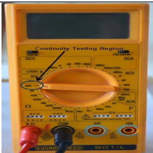
Fig. 3.16: Continuity Test using Multi meter
