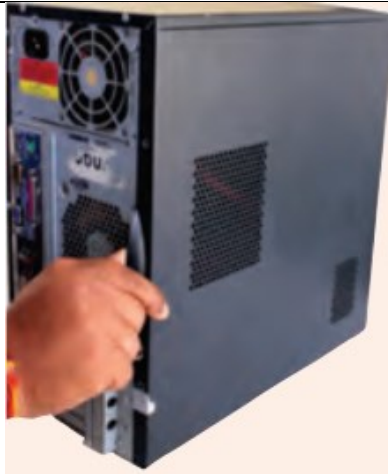
Fig. 1.10 Remove the side panel
